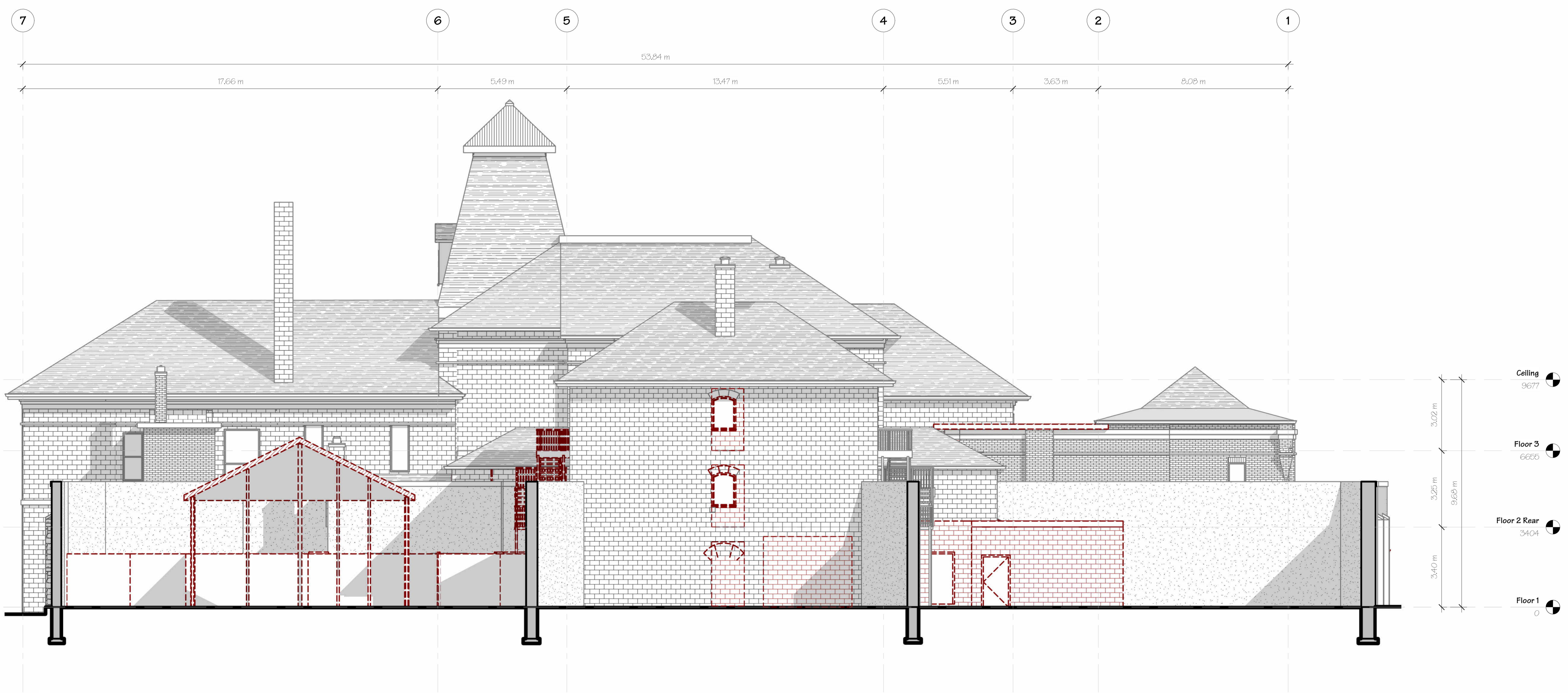
1 COURTYARD EAST ELEVATION - EXISTING & DEMOLITION 1:75
